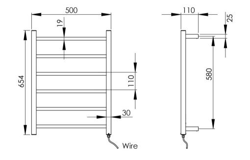
Electricity Input: 240V, 50Hz | Power Rating: 62W | IP Rating: IPX5 | Connection position: Bottom right | Connection type: Plug-in or Hardwire
