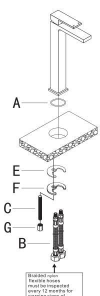
Braided nylon flexible hoses must be inspected every 12 months for warning signs of failure including bulging, rust spots, wear, moisture, snapped threads, kinking, water staining, general corrosion or discolouration. Mixer tails showing any signs of the above mentioned warning signs must be replaced immediately.
