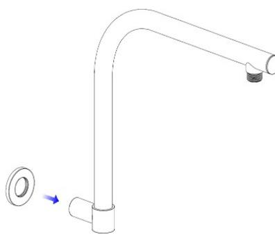
2. Push on cover plate and screw on wall arm
