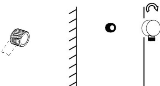
4. Attach hose to water supply elbow and hand shower. Fit the hand shower into slider bracket.
