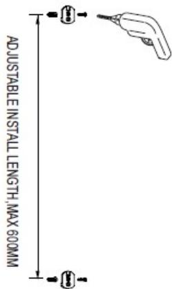
2. Fit slider bracket and fixing posts to rail and attach to base supports on wall.
