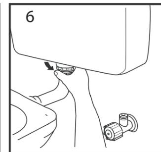
6 Hand tighten the coupling nut.
