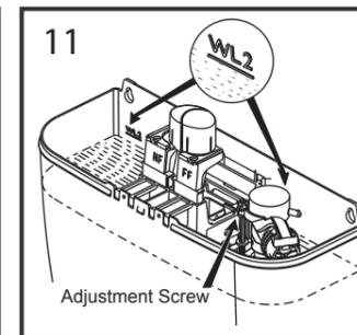
11 Actuate the Inlet valve at least once to purge any trapped air in the valve. Adjust the water level to the WL2 mark.
