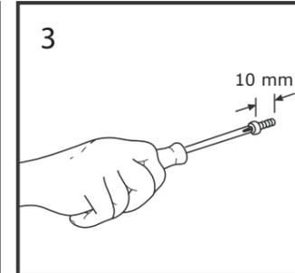
3 Leave the screws protruding by 10mm.
