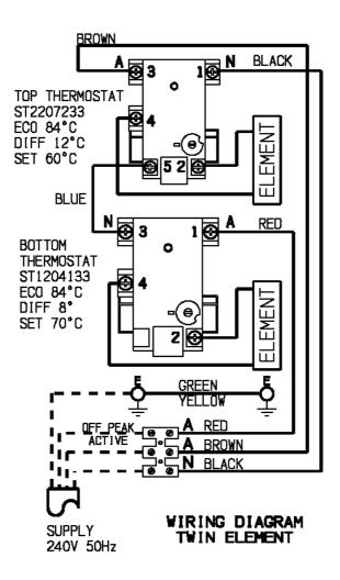
Top thermostat – fixed setting Bottom thermostat – tradesperson adjustable 60°C. min 60°C, max 75°C.
