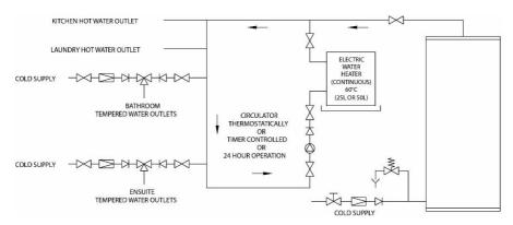
Circulated Hot Water Flow and Return - Off-Peak Electric Water Heater
