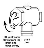
⚠ **DANGER:** Failure to operate the easing lever on the relief valve once every six (6) months may result in the water heater cylinder failing, or under certain circumstances, exploding.
