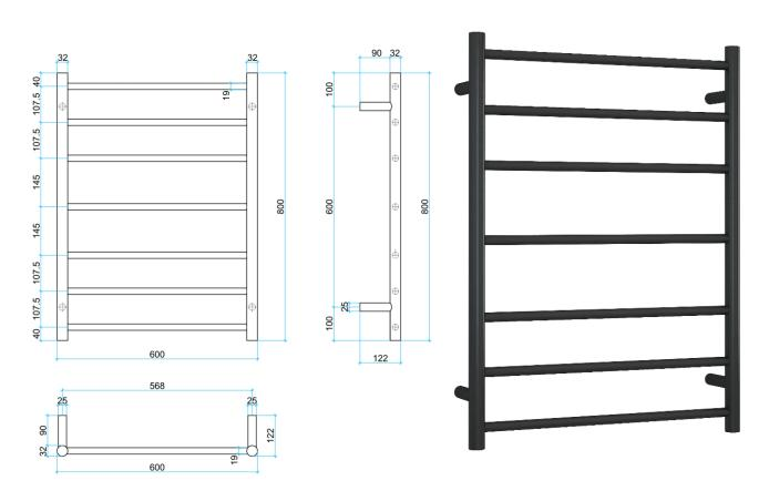
This rail has Multiflex wiring which means that there is a connection point on both the left and right hand side of the rail and the lead can be connected to either side. Being a dry electric element rail, this can be mounted either way up meaning the wiring can be from any of the four mounting points.
