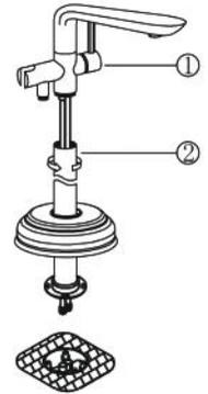
9. Fix pipe in N-box, adjust position, fix panel by M5 screw.
