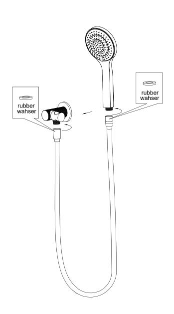
4. Connect bracket and hand shower with hose. TEST & CHECK FOR LEAKS.
