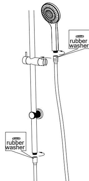
6. Please noted the rubber washer in the hand shower. Connect shower rail and hand shower with hose. TEST & CHECK FOR LEAKS.
