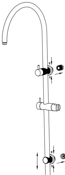
4. Locate and push shower rail assembly onto wall adaptors. Tighten grub screws firmly with allen key provided. Slide the back plates against the wall/tile face properly.
