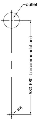
1. Drill a  $\phi 6$ mm hole at the downwards outlet vertical downward position in the recommendation range.
