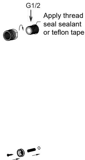
2. Screw the adapter onto the outlet. Push wall plug into drilled hole. Fit lower mounting pillar in place with screw. Tighten firmly.
