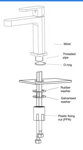
1. Fit the O-ring into the groove in the underside of the mixer body.
