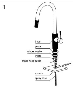
Use a 35mm hole saw cut a hole through the counter. Remove the lock nut, triangle plate, steel washer. Feed spray hose through the hole and position the mixer over the hole.
