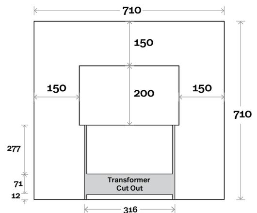
All measurements are in 'mm' and are approximate and to be used as a guide only. Installation preparations are not recommended without product onsite.
